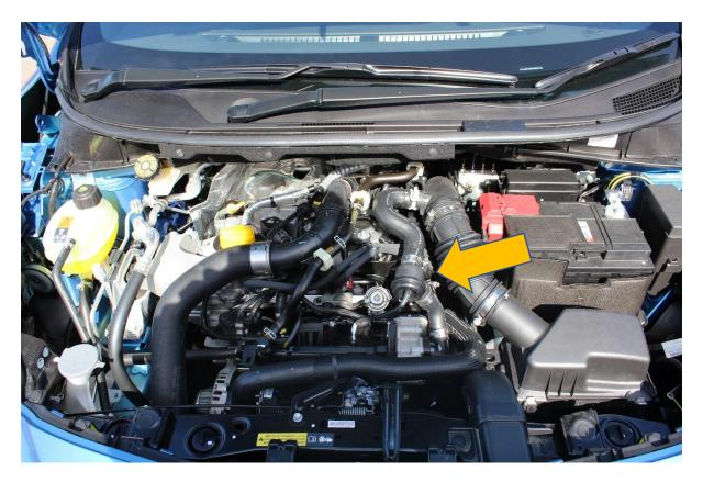
2. Remove the vacuum line from the top of the valve. Using a hose clamp drive, loosen the remaining hoses and remove the OEM valve.
